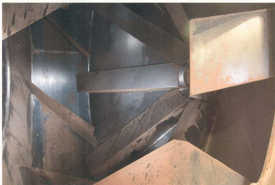
Mixing flights inside the mixer's rotating drum lift, cut, fold, and tumble the material to achieve complete blend uniformity.
